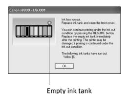
The ink tank with [X] symbol is out of ink. Replace with a new ink tank.
